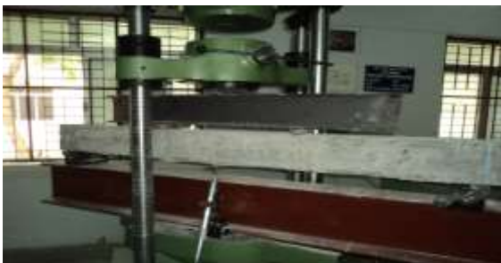
Fig 3: Two point loading for RC beams
